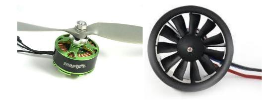
The propeller method provides more lift, a more linear throttle-thrust response, and better efficiency at low throttle. However, the propeller's required space is large and puts a minimum size constraint on SDP design.
