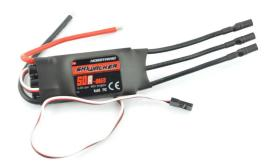
The final choice is the SkyWalker 50A BEC, though the specific model does not matter. Any standalone 50A esc would suffice.
